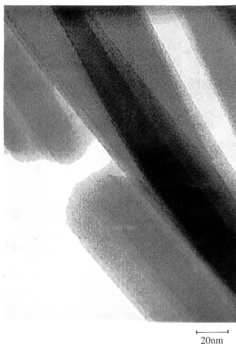
Fig. 7 TEM images (500 000 × magnification) of the reaction product of \text{Zn}(\text{OH})_2 with benzoyl chloride.
